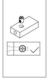
Please ensure that the threaded hole of the horizontal nut is aligned with the horizontal hole at the end of the wooden board, otherwise the screw cannot be installed
