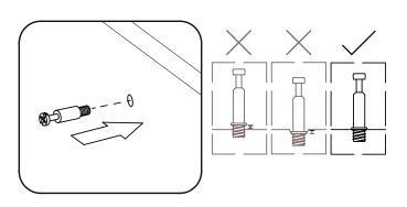
Next, you will fit the proper hole on the edge of the associated joining panel over the cam bolt.
