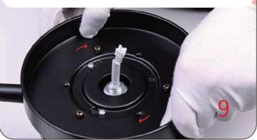
9. Insert the third light kit screw, and then tighten all three light kit screws
