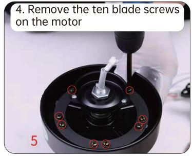
and loosen the two light kit screws pre-locked on the motor (They will be needed later.)
