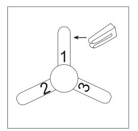
Slide the balancing clip on the trailing edge of any blade, halfway between the holder and tip. Run the fan to check the wobble. If the wobble persists, repeat with each blade, noting which one most reduced the wobble.
