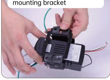
45. Install the ceiling bracket with four self tapping screws.(Is your ceiling different? Check out the guide at the page of 3.)
