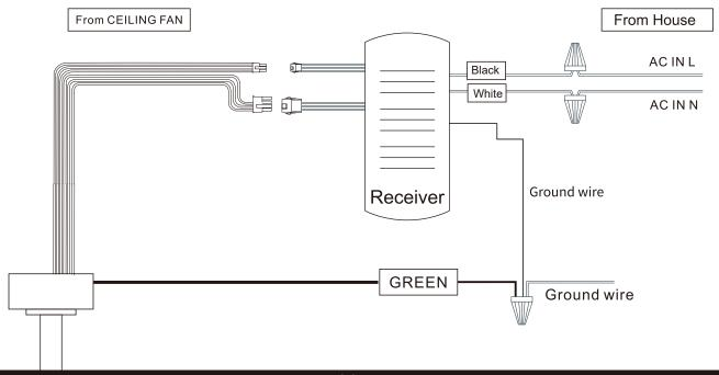
30. Connect the wire from the ceiling fan to the receiver( Red, White, and Black wires)
