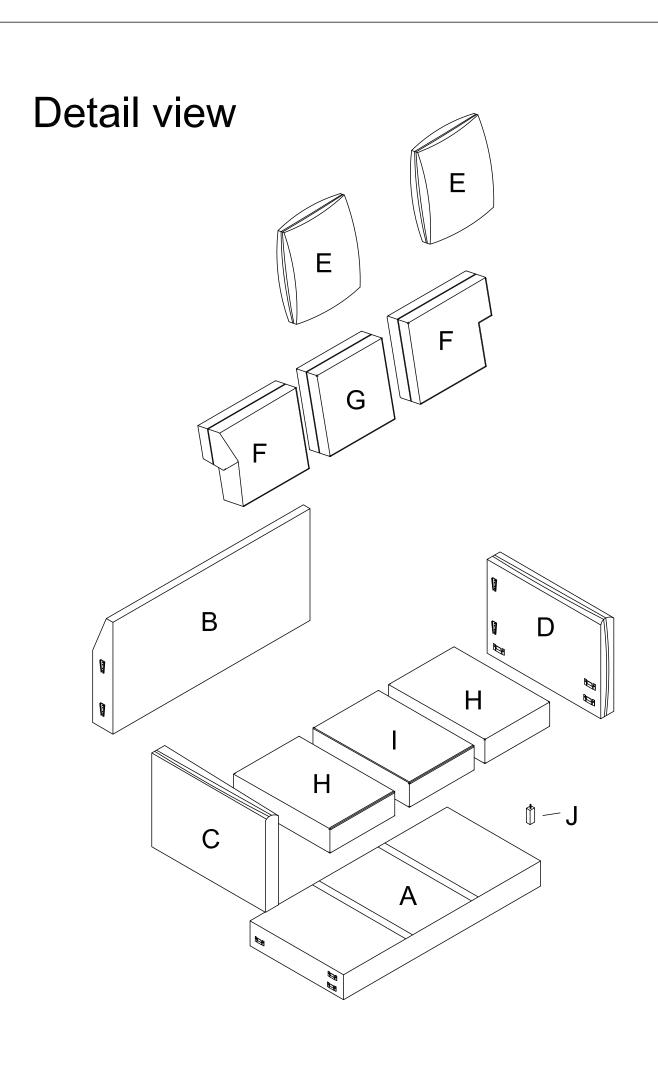
Step 1; Assembling Arms (C and D) to the seat (A) as shown.
