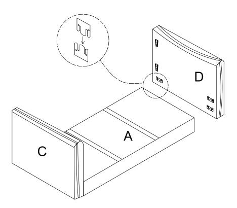
Step 2; Assembling Back (B) to the Arms and Seat (C and D) as shown.
