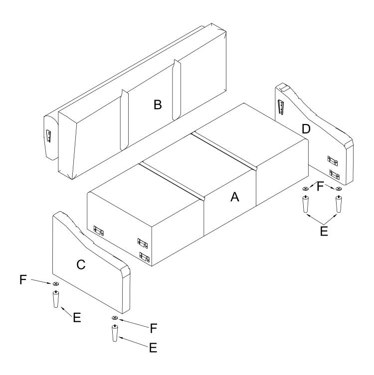
Step 1; Screw four legs (E) through washers (F) into the bottom of Arrms (D and C) as shown.
