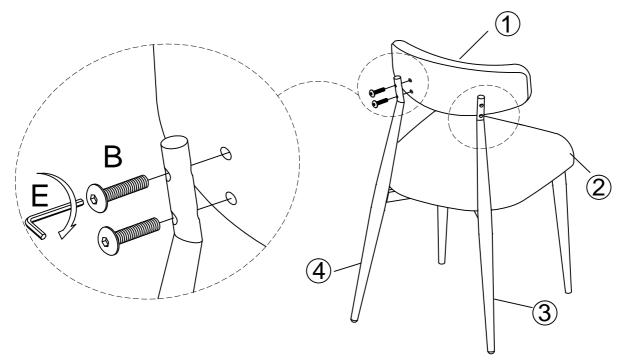
Note: Do not fully tighten the bolts at this step.
