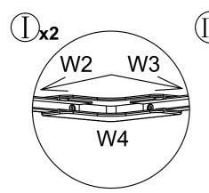
Insert the other end of W2 and W3 into corner guard W4.
