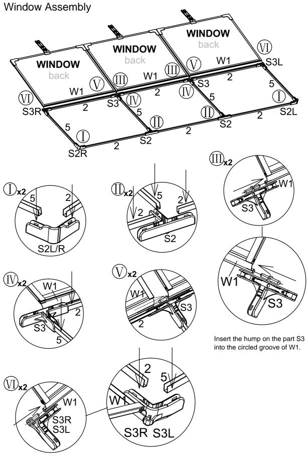
Insert the hump on the part S3R and S3L into the circled groove of W1.
