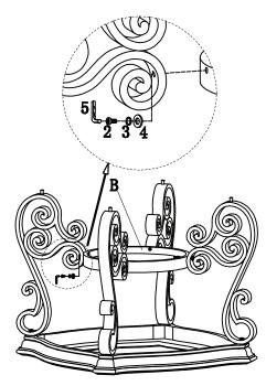
STEP 2: Attach Shelf (B) to Legs (E) by using Allen Key M4 (5), Allen Bolt 1/4" x1"28mm (2), Spring Washer 1/4" (3), Flat Washer 1/4" (4)
