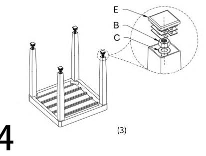
**Step 4**: Do not over tighten bolts, it will cause the damage of product without warranty;Your table should be ready for use. If your table is not stable, double check your assembly procedure or loosen some bolts and tighten them again.
