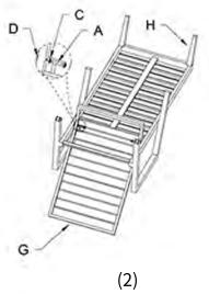
**Step 3**: Adjust the **Seat(H)** and **Back Panel(G)** to the appropriate Angle .Install hardware parts(**B**) in order displayed as Fig(3) and connect the gas rod to the backrest use **Allen Wrench(F)**.
