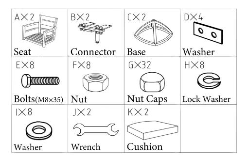
Step 1:Place all the parts on a clean and soft surface, identify all the parts and hardware kits against parts list. Assemble **Seat(A)** and **Connector(B)** first, and make sure the direction of **connector(B)** is correct as Fig(1). This is very important for safe.
