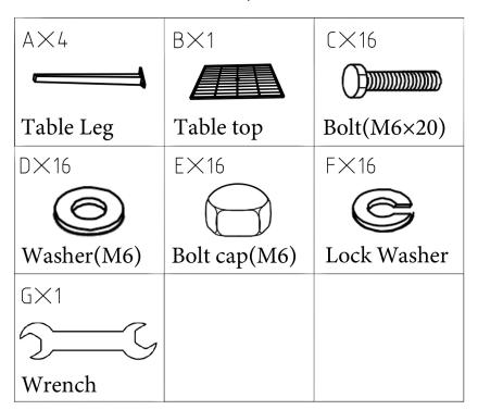
Step 1: Place all the parts on a clean and soft surface, identify all the partsand hardware kits against parts list. Turn over the Table top(B) onto a flat surface. Attached Table Legs(A) with parts (D,F,C,E) to the Table top(B) pre-installed by manufacturer on the seat as Fig1 and tighten all bolts.
