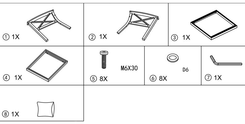
**Step 1:** Install Part 1(Leg) and Part 2(Leg) to Part 3(Seat) with Part 5(Screws) and Part 6 using Part 7(Wrench).
