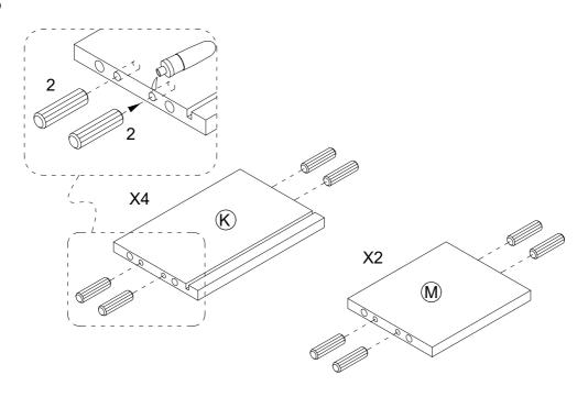
Glue the wood dowels 2 into the inner holes on the front upper rail K and M . NOTE: It is very important to use a small amount of glue 10 on ends of dowels and wipe away excess glue immediately.
