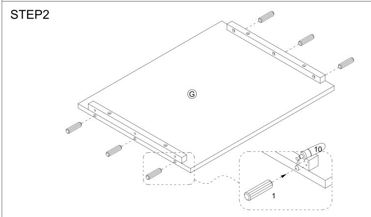
Glue the wood dowels 1 into the inner holes on the side panels G. NOTE: It is very important to use a small amount of glue 10 on ends of dowels and wipe away excess glue immediately.
