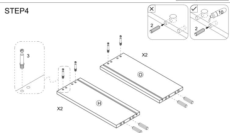
Glue the wood dowels 2 into the inner holes on the front upper rail H and O . NOTE: It is very important to use a small amount of glue 10 on ends of dowels and wipe away excess glue immediately.
