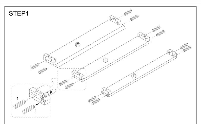
Glue the wood dowels 1 into the inner holes on the front upper rail D ,E and F . NOTE: It is very important to use a small amount of glue 10 on ends of dowels and wipe away excess glue immediately.
