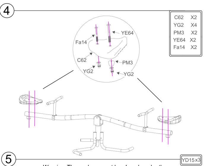
Warning: The anchors must be placed under the ground in order to reduce tipping hazards
