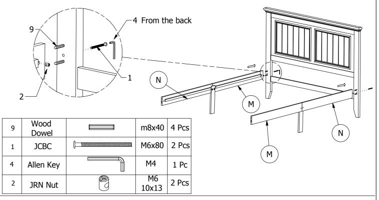
Step 11: Pre-insert Wood Dowel (9) on the Footboard Posters (G / H). Take Side Rail (M & N) to push in to the wood dowel. Then put in the JRN Nut (2) on the pre-drilled hole and use JCBC (1) to tighten- screw from the front of footboard posters. This assembly step is using the Allen Key (4).
