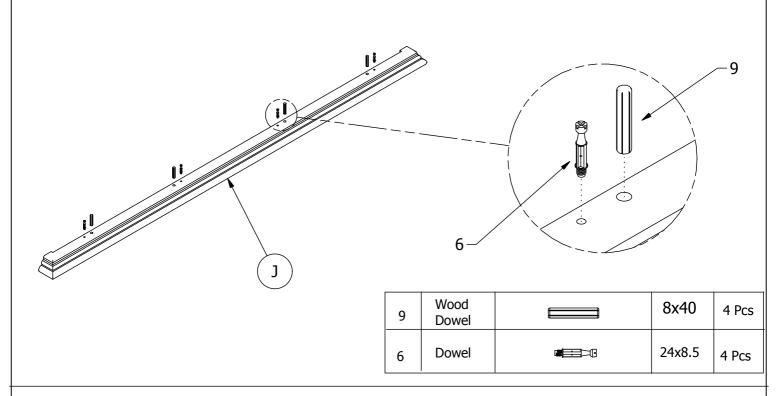
Step 6: Push-attach the Headboard Top Cap (J) into the headboard panel part assembled earlier. Then tighten the connection with Ultra Shallow Cam (5), you will need to prepare a screwdriver.
