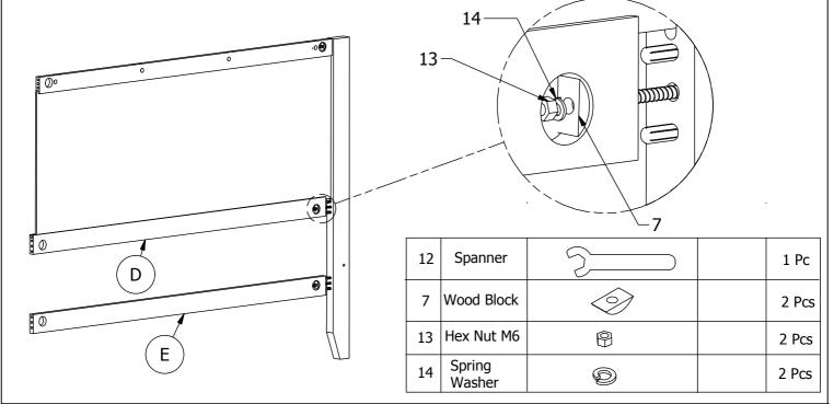
Step 4: One side of Headboard Bedpost with Headboard Panel is ready.... attach it with Headboard Bedpost-R (L). Repeat the assemble step like previous steps above.
