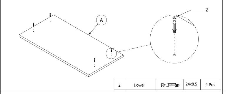
Step 4: Ready the cabinet structure and flip the Table Top (A) to cover on top of the cabinet. Then tighten the attachment with Ultra Shallow Cam (3) to the Dowel pre-installed in previous step 3. You would need to ready a screwdriver to perform this step.
