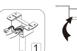
\* Selection of hanger pipes I. Use hanger pipes at an appropriate height based on the height of the ceiling. 2. This ceiling fan is provided with the hanger pipe at the length of 10 inches and 20 inches. \* The bottom of the fan lamp must be ensure 2.3 meters
