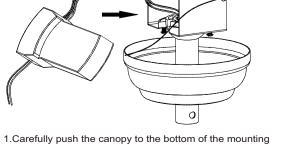
bracket, make two sliding holes aligned to the two prominent screws on the mounting bracket, and then turn clockwise 2. Push the canopy ring to the bottom oft he canopy, slide the inner holes aligned to the two prominent screws on the mounting bracket again, and turn the canopy ring clockwise until tight.
