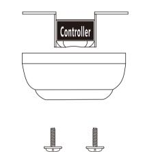
Remove and save the two canopy screws in the round holes.
