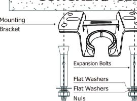
For concrete ceiling, use the percussion bit with diameter 8mm to drill holes according to the length of expansion screws. Then use the attached expansion screws to fix the hanging bracket onto the ceiling (selection is made according to actual requirements of the customers).
