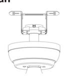
☐ Lift the fan motor assembly up to the mounting bracket and seat the hanger ball in the mounting bracket socket.Rotate the fan motor assembly until the check groove drops into the registration slot and seats firmly. The downrod should not rotate if the is done correctly
