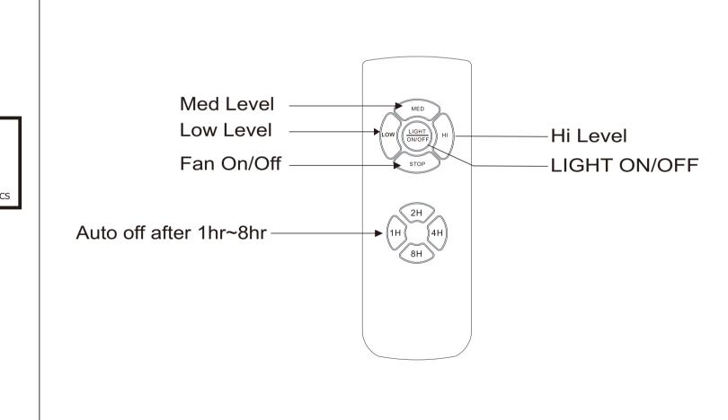
LOW FanSpeed Low Level MED FanSpeed Middle Level
