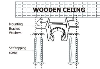
For wooden ceiling, use wood screw to drill on the wooden beam or the "junction box" to fix the hanging bracket(selection is made according to actual requirements of the customers)
