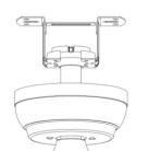
☐ Lift the fan motor assembly up to the mounting bracket and seat the hanger ball in the mounting bracket socket.Rotate the fan motor assembly until the check groove drops into the registration slot and seats firmly. The downrod should not rotate if the is done correctly
