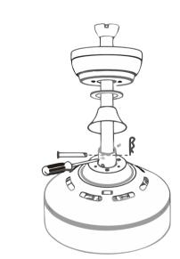
☐ Align the holes and replace hanger pin and locking pin.
