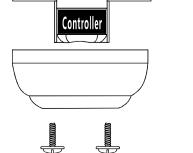
I:Remove the mounting bracket from the canopy by loosening the two canopy screws located in the L shaped slots 2:Remove and save the two canopy screws in the round holes.
