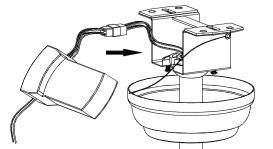
1. Carefully push the canopy to the bottom of the mounting bracket, make two sliding holes aligned to the two prominent screws on the mounting bracket, and then turn clockwise 2. Push the canopy ring to the bottom oft he canopy,
