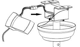
1. Carefully push the canopy to the bottom of the mounting bracket, make two sliding holes aligned to the two prominent screws on the mounting bracket, and then turn clockwise 2. Push the canopy ring to the bottom oft he canopy,
