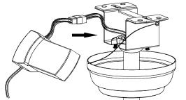
1. Carefully push the canopy to the bottom of the mounting bracket, make two sliding holes aligned to the two prominent screws on the mounting bracket, and then turn clockwise 2. Push the canopy ring to the bottom oft he canopy, slide the inner holes aligned to the two prominent screws
