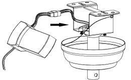
1. Carefully push the canopy to the bottom of the mounting bracket, make two sliding holes aligned to the two prominent screws on the mounting bracket, and then turn clockwise 2. Push the canopy ring to the bottom oft he canopy, slide the inner holes aligned to the two prominent screws on the mounting bracket again, and turn the canopy ring
