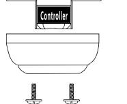
I:Remove the mounting bracket from the canopy by loosening the two canopy screws located in the L shaped slots 2:Remove and save the two canopy screws in the round holes.
