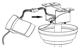
1. Carefully push the canopy to the bottom of the mounting bracket, make two sliding holes aligned to the two prominent screws on the mounting bracket, and then turn clockwise 2. Push the canopy ring to the bottom oft he canopy, slide the inner holes aligned to the two prominent screws
