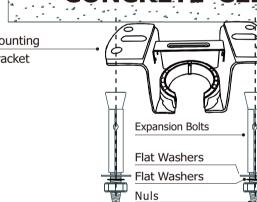
For concrete ceiling, use the percussion bit with diameter 8mm to drill holes according to the length of expansion screws. Then use the attached expansion screws to fix the hanging bracket onto the ceiling (selection is made according to actual requirements of the customers).
