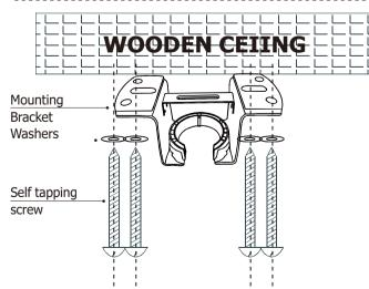
For wooden ceiling, use wood screw to drill on the wooden beam or the "junction box" to fix the hanging bracket(selection is made according to actual requirements of the customers)
