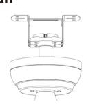
☐ Lift the fan motor assembly up to the mounting bracket and seat the hanger ball in the mounting bracket socket.Rotate the fan motor assembly until the check groove drops into the registration slot and seats firmly. The downrod should not rotate if the is done correctly
