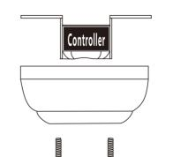
1:Remove the mounting bracket from the canopy by loosening the two canopy screws located in the L shaped slots. 2:Remove and save the two canopy screws in the round holes. This will enable you to remove the mountingbracket
