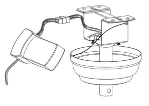
Carefully push the canopy to the bottom of the mounting bracket, make two sliding holes aligned to the two prominent screws on the mounting bracket, and then turn clockwise
