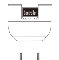
Remove the mounting bracket from the canopy by loosening the two canopy screws located in the L shaped slots. Remove and save the two canopy screws in the round holes. This will enable you to remove the mountingbracket
