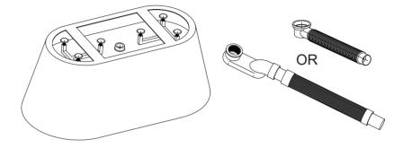
4 Turn the bath the right way up and rest on two blocks(ideally4"x4")in position to gain access underneath to attach the household pipework.
