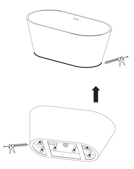
Please allow 24 hours for the silicon to dry off before use. The installation guide includes options for waste connection: The final decision about installation and waste connection should be taken by a qualified person.
