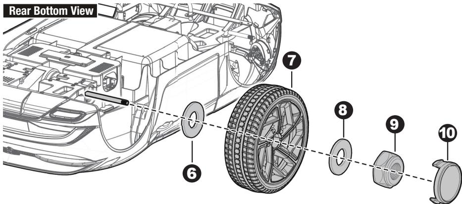
6. Slide the  $\varnothing 10$  washer onto the rear axle (Right Side).
