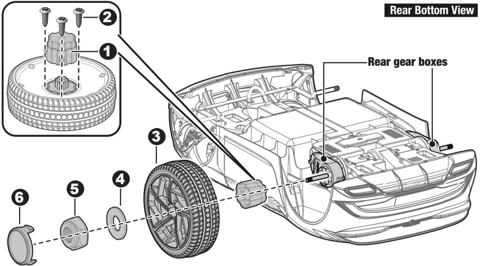
Remove all the parts from the rear axle.
