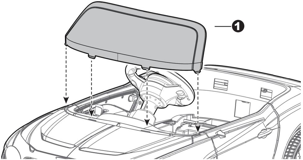
1. Fit the tabs windshield into the grooves on the vehicle. Press until you hear it “click” into place.
