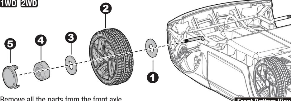
Remove all the parts from the front axle.
