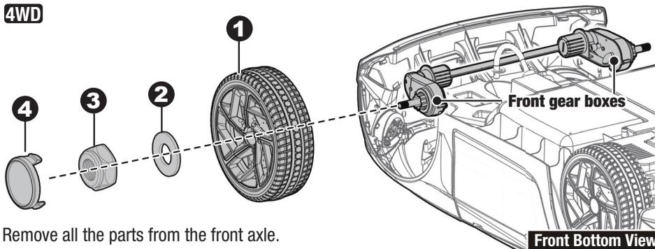
Remove all the parts from the front axle.
