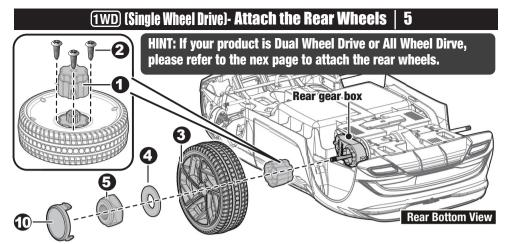
Remove all the parts from the rear axle.
