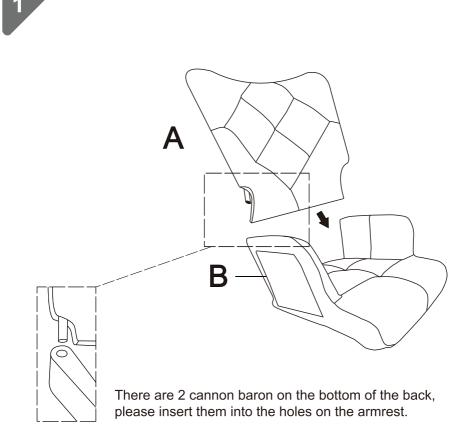
Attention : 1.screws should be only 50% tight. 2.after all the screws adjust the holes then tight screws 100% totally.
