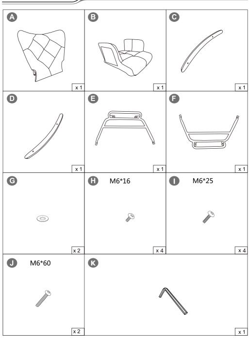
Attention : 1.screws should be only 50% tight. 2.after all the screws adjust the holes then tight screws 100% totally.
