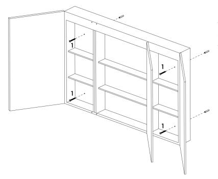
**Note:** When mounting to the wall, the wire can not be pressed between the cabinet and the wall, otherwise the wire installation will be affected.
