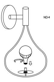
5. Finally, put the glass lampshade over the bulb and tighten it  $${\rm N}{\sc \Box}{:}5$$
