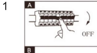
Please confirm whether the voltage is consistent with the product, and turn off the power supply at the installation position to ensure safety.
