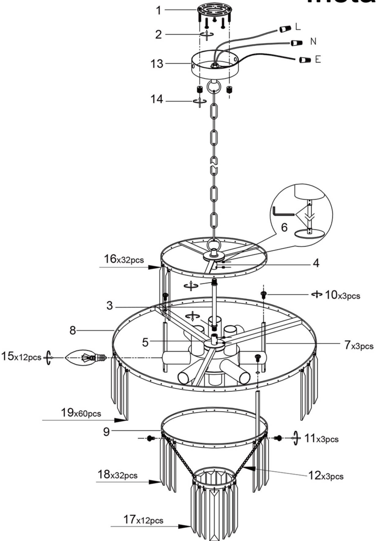
I: Use screws(2) to fasten the metal bracket(1) on the ceiling.
