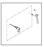
STEP 03: Use impact drill punch holes in the marked center (6-8MM drill bit), the drilling depth is about 5CM. Use a hammer to drive the expansion screw into the drilled hote.
