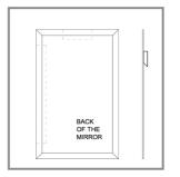
STEP 01: Check the wall.Make sure that the wall is bearing walls that can support the Mirror's weight. Measure the width and height of the mirror back holes/hocks distance with a tape measure.
