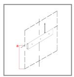
**STEP 02:** Mark the punching position on the wall with a pencil. Use level gauge make sure the hole at the same level.
