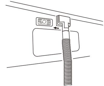
Use a screwdriver to fix the screw on the edge and strengthen the drain pipe;
