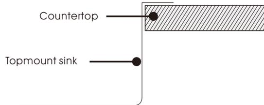
**2** Cut out the appropriate template for your sink model and desired installation option. Place template in desired position on countertop , locating center of the bowl over cabinet and faucet holes. Trace the line of the template and cut countertop according to templated size. using appropriate cutting tools. Template is for guide only. Use physical sink to ensure accurate cutout opening.
