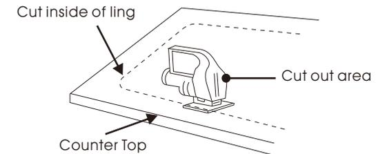
**3** Cut out the appropriate template for your sink model and desired installation option. Place template in desired position on countertop , locating center of the bowl over cabinet and faucet holes. Trace the line of the template and cut countertop according to templated size. using appropriate cutting tools. Template is for guide only. Use physical sink to ensure accurate cutout opening.
