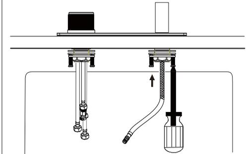
Push the quick connector firmly upward and attach it to the receiving block. Pull down moderately to ensure the connection has been made. Install the Weight & Clip Assembly.
