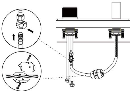
Thread the nut on the supply line onto the outlet of the water supply valve and tighten with a wrench. Do not overtighten.
