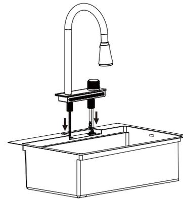
Install the rubber washer and metal washer onto the threaded mounting shank. Thread the nut onto the mounting shank. Lock the nut into position by tightening the screws. Do not overtighten.
