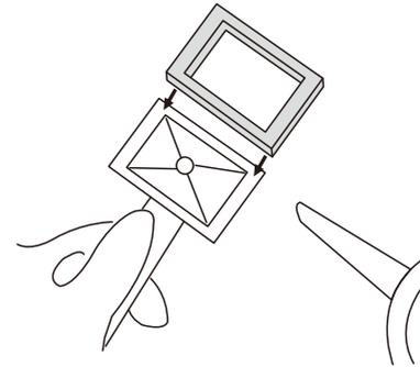
The drain pipe is aligned with the opening of the sink, pay attention to the screw hole of the drain pipe.
