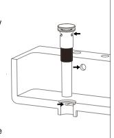
1 Unscrew components A & B to the seal.
