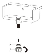
4 Connect the rear end of the drain to the Drain Pipe.
