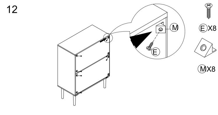
Put hardware M to the groove and tighten them with hardware E .
