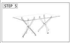
Attention: When assembly is complete, set the table upright on its base. With at least 2 people, carefully lift the table up from underneath and rotate onto the base Caution:
