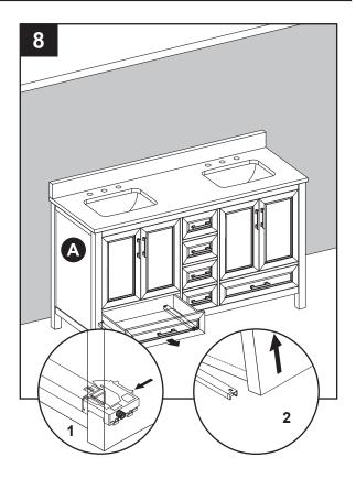
9. To reinstall drawer(s) into vanity (A), fully extend metal glide tracks. Gently lower and slide drawer box into rear glide catch. Next, lower drawer box down to completely rest on extended glides. Then, push plastic levers to lock the drawer box in place.
