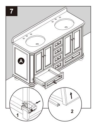
8. To reinstall drawer(s) into vanity (A), fully extend metal glide tracks. Gently lower and slide drawer box into rear glide catch. Next, lower drawer box down to completely rest on extended glides. Then, push plastic levers to lock the drawer box in place. Repeat for remaining drawers
