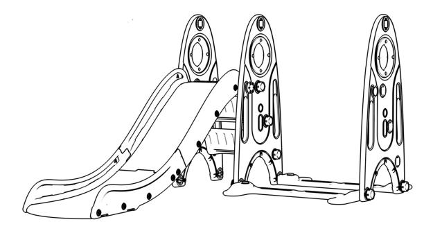
2. Attach the other Part D to the 2 Part F, secure with 2 Screw e.
