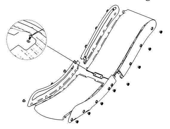
**1**. Connect the Part B to the Part A, secure with 2 Screw g.
