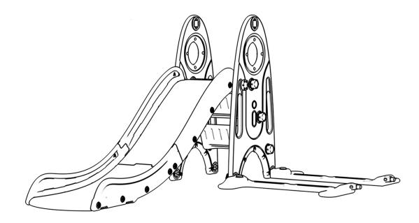
Attach the 2 Part F to the Step 2 assembled parts, secure with 2 Screw e.
