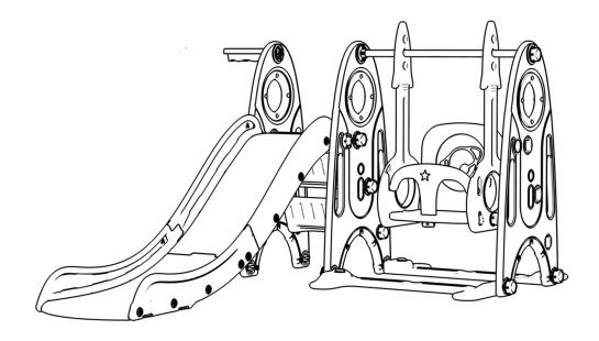
Connect the Step 4 assembled parts to the Step 3 assembled parts, secure with 2 Screw e.
