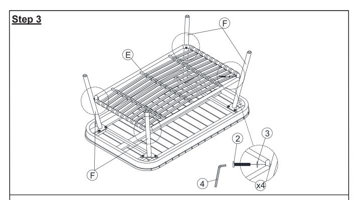
From step 2, Using the Allen Key (4), attach Shelf (E) into Leg (F) as shown above by using Bolts (2) and Washer (3). Fully tighten the Bolts.
