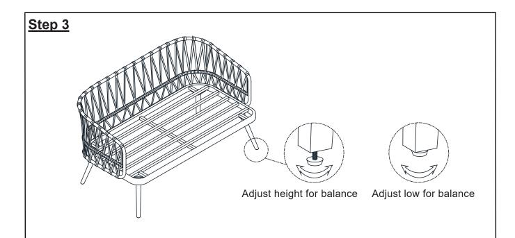
In a sequential manner, tighten all Screws and Bolts at all joints.
