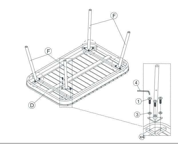
With assistance from your adult partner, please carefully upside down Table Top (D). Insert four Leg (F) to Table Top (D) by using Bolts (1) and Washer (3) as shown in the above picture. Do not fully tighten the Bolts.
