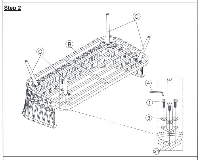
With assistance from your adult partner, please carefully upside down Seat Frame (B). Insert four Leg (C) to Seat Frame (B) by using Bolts (1) and Washer (3) as shown in the above picture. Fully tighten the Bolts.
