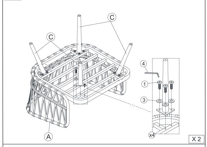
With assistance from your adult partner, please carefully upside down Seat Frame (A). Insert four Leg (C) to Seat Frame (A) by using Bolts (1) and Washer (3) as shown in the above picture. Fully tighten the Bolts.
