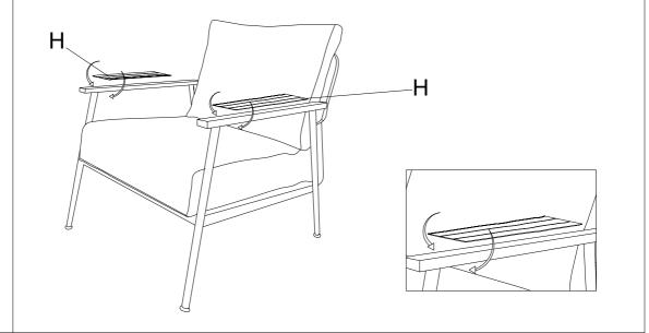
Next, put on Armchair's Fabric (H) on the both side of arm chair. Make sure both of Armchair's Fabric (H) are fit neatly.
