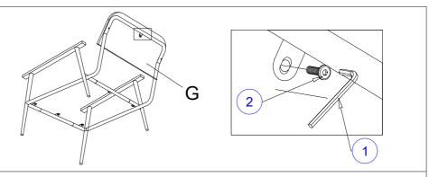
Next, attach Back Rest Board (G) to the Metal Top (A). Align the mounting positions on the Back Rest Board (G) and Metal Top (A). Lock in the middle mounting position, using Bolt (②) and Allen Wrench (①).
