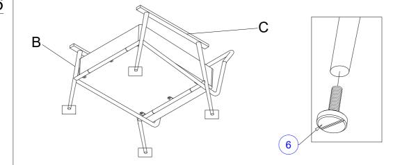
Mount Stopper (ⓐ) at the bottom of Metal Leg Left (B) and Metal Leg Right (C). Use your hand to tighten Stopper (⑥).
