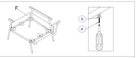
Attach Cushion Seat (F) to the Metal Support (D), Metal Leg Right (C) and Metal Leg Left (B). Align the mounting positions on the Cushion Seat (F) with Metal Leg Left (C), Metal Leg Right (B) and Metal Support (D).
