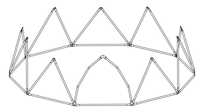
**Note:** Each joint at the bottom circle is connected by 4 tubes.
