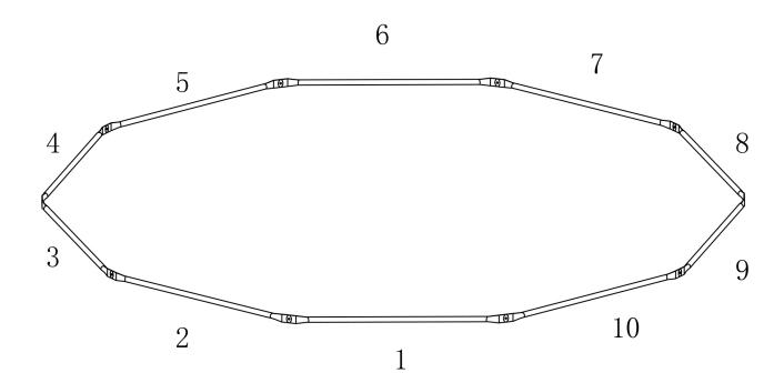
Slide an M8 Washer(8#) over M8 x 30mm Bolt(7#), then slide the Bolt(7#) through the joint of 2pcs White Tubes(1#) on the ground, 1pc Blue Tube(2#) and 1pc White Gate Tube(4#) in the order indicated by the numbers. Secure Bolt(#7) with an M8 Nut(#9).
