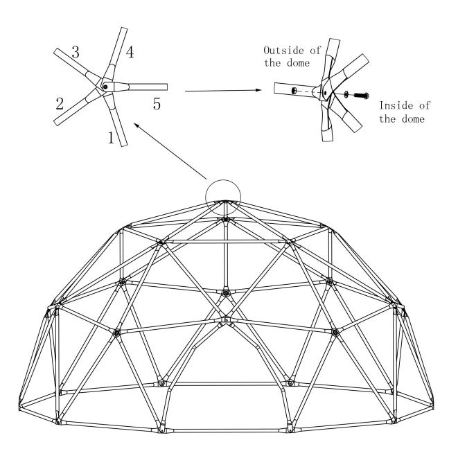
Install the Climbing Grips to cover the bolt on each of the joint. Small Climbing Grips (10 pcs) should be installed on the bottom joints. Large Climbing Grips (16 pcs) should be installed on the joints not touching the ground.
