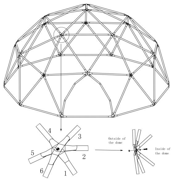
Secure the joint on top with 1pc M8 x 30mm Bolt(7#), 1pc M8 Washer(8#) and 1pc M8 Nut(9#).
