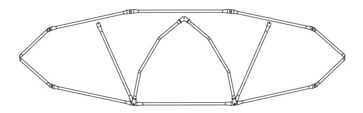
Repeat the same step to attach a Blue Tube(2#) and a White Tube(1#) to the next joint, and secure with 1pc 8 x 30mm Bolt(7#), 1 pc M8 Washer(8#) and 1pc M8 Nut(9#).
